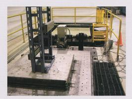
MET's seismic test systems can accommodate large cabinets or multiple rack systems. MET employs a high performance value that allows ETSI / NEBS operational shock and vibration profiles on one shaker, saving significant time by not having to switch from a hydraulic to an electro-dynamic system. Installation set-up includes an electric overhead crane for the safe and efficient movement of test systems.
