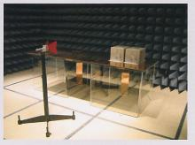
MET is one of a few labs that can test 200 V/m **Radiated Immunity and EMP** testing per MIL-STD-461/462 in-house.
